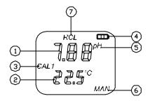
Main display - 3½ digit display providing direct readout of pH. Underrange (-1) and Overrange (1) symbols will be displayed if the instrument is reading outside the ranges of:
